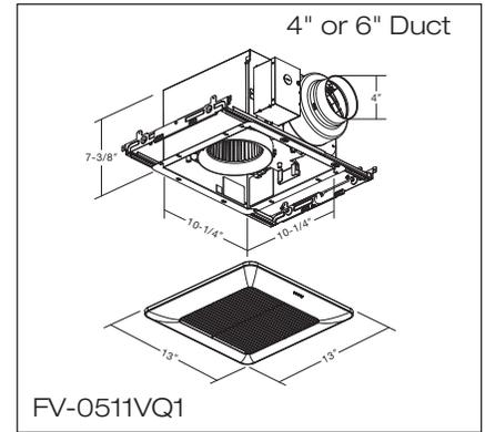
run continuously. ECM motor speed shall automatically increase when the fan senses static pressure to maintain selected CFM. Power rating shall be 120V/60Hz. Duct diameter shall be no less than 4", inclusive of an integrated dual 4" or 6" duct adapter. Fan can be used to comply with ASHRAE 62.2, LEED, ENERGY STAR® IAP, EarthCraft, CA Title 24 and WA state code.
