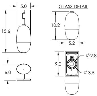
Mounting Method: J-Box Wall Mount. **Minimum J-Box Size Requirement is 4" W, 4" L, 1.5" D**
