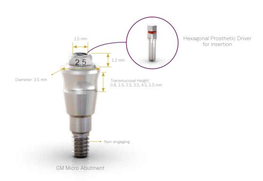
Note: The GM Micro Abutment can be used for crowns or multiple prostheses. It is not available with different angles.
