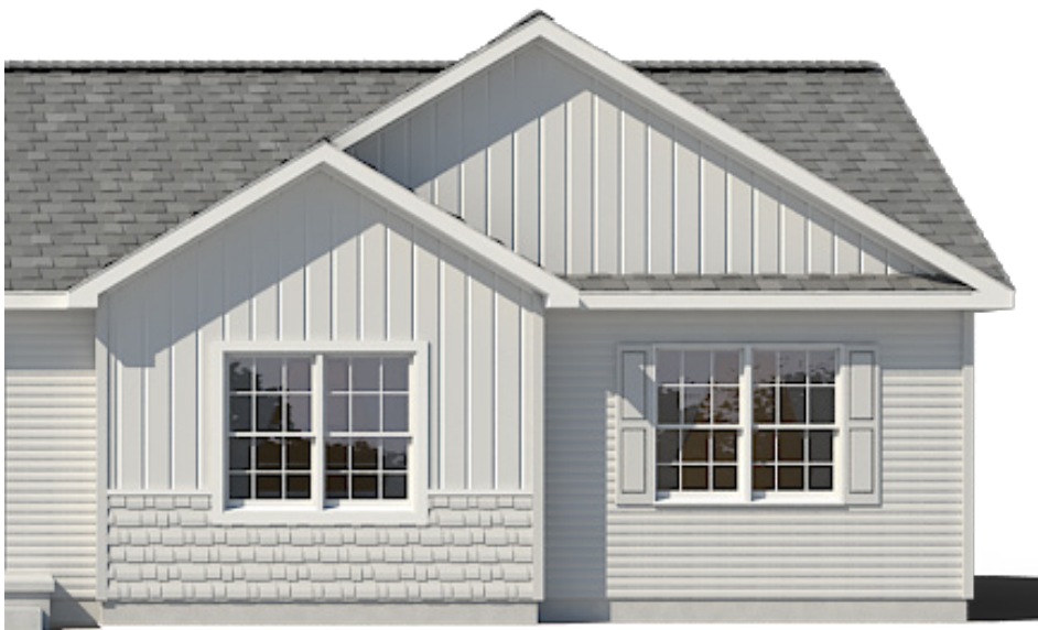
27'-4" or 22' Twin Peak Dormer with Bump-out 5/12, 7/12, 9/12 & 12/12
