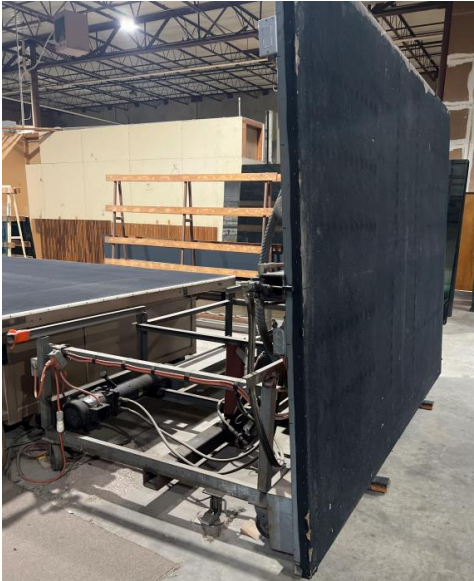
Break out table with breaker bars and air float. With 5 120v outlets. 9' x 11'10"
