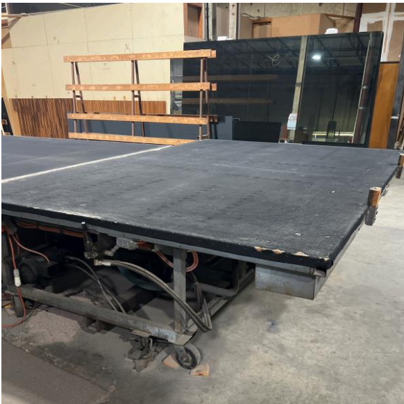
Break out table with breaker bars and air float. With 5 120v outlets. 9' x 11'10"
