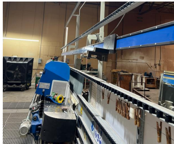
Bovone ELB-14 with custom welded extension rack and pad scrubbers. Flat polish 1/8 to 1". Also has clip corner clamp rail system (powder coated Bovone blue). $110,000
