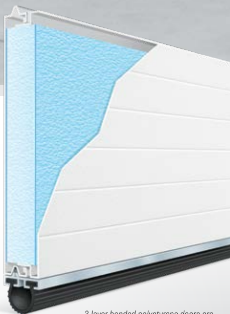
3-layer bonded polystyrene doors are 2" or 1-3/8" sandwich construction
