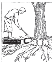
Figure 2. Placement of this product as a soil injected treatment
