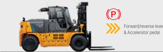
Auto hold: Automatically engages parking brake when brake pedal is held for more than four seconds. Auto parking: Automatically engages the parking brake when the operator leaves the seat.
