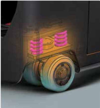
Driver Impact Reduction By applying a spring damper to the floorboard and adding a spring on the caster wheel, driver impact is reduced in rough or uneven work environments, providing improved comfort.
