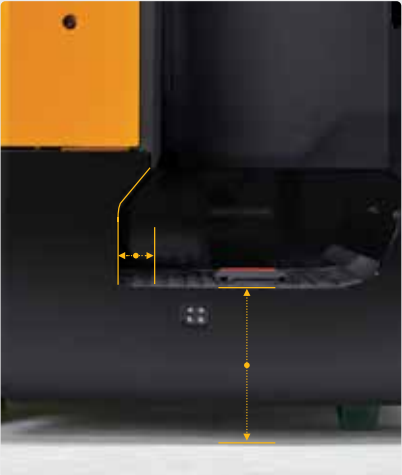
Additional Toe Space & Lower Step Height The additional toe space allows operators to naturally position their feet, reducing strain on the legs during long shifts. The step height has been lowered to just 10.6" for ease of entry.
