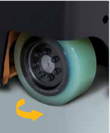
Auto Drive Tire Centering Upon start up, the drive tire automatically centers, ensuring the truck is not starting with the drive tire at an angle, which also contributes to a safer operating environment.
