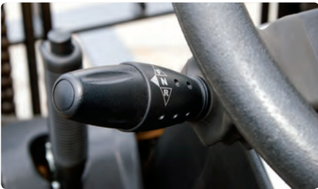
Easy and Safe Shift Lever A single lever on the left side of the steering column gives the operator fast, easy control of direction. The lever must be in the neutral position before the engine can be started.
