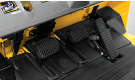
Ergonomically Positioned Pedals Based on human engineering, the accelerator, brake and inching pedals are optimally positioned for convenience while operating the equipment.
