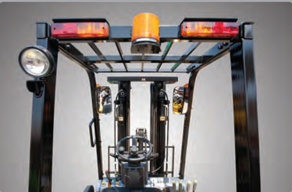
New High Visibility for Safe Operation The operator is able to work with increased safety and accuracy due to a wide view through the mast, standard mirrors and spacious compartment.
