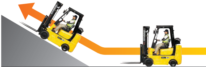
Increased Mast Tilting Angle Utilizing the mast tilting angle of 6 degrees forward and 8 degrees backward, the operator can safely and rapidly perform loading and unloading jobs.
