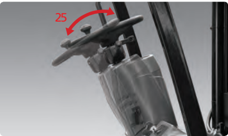
Adjustable Steering Wheel Steering wheel with horn button can be adjusted by a lever on the right-hand side for the most comfortable operator position.
