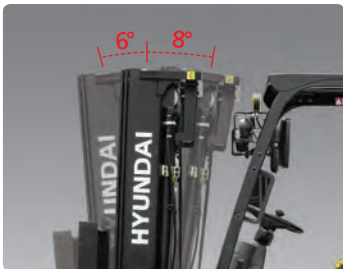
Increased Mast Tilting Angle Utilizing the mast tilting angle of 6 degrees forward and 8 degrees backward, the operator can safely and rapidly perform loading and unloading jobs.
