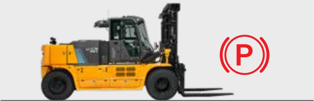
Auto hold: Automatically engages the parking brake when the brake pedal is held for more than four seconds. Auto parking: Automatically engages the parking brake when the operator leaves the seat.
