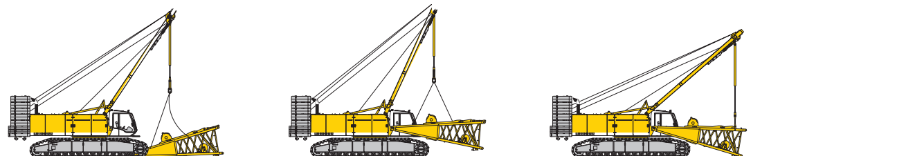
Unloading and assembly of boom foot
