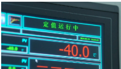
HMI display Low-temperature performance test under -40 °C
