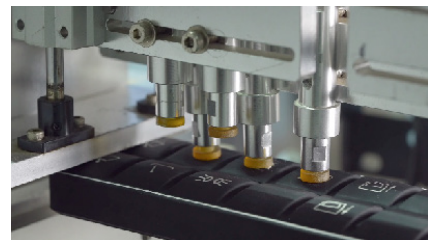
Panel buttons cycled 1.2 million times
