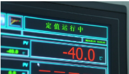
HMI display Low-temperature performance test under -40 °C
