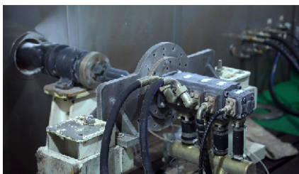
Hydraulic pump undergoing Low-temperature performance test under -40 °C
