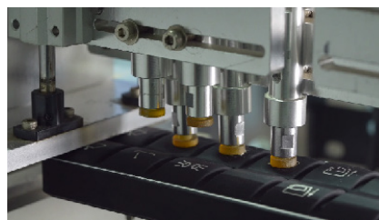
Panel buttons cycled 1.2 million times
