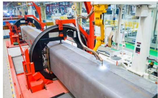
UNMANNED AUTOMATIC WELDING
