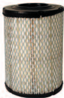
Air Filter, Club Car Gas 84-91 Paper element with wire mesh encasement and sealed ends. OEM: 1012506; 1013379. FIL-0005
