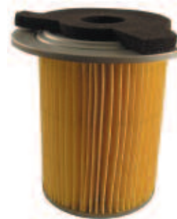
Air Filter, Yamaha G1 2 Cycle Gas 78-89 and G14 4 Cycle Gas Oil treated paper element with O-ring top seal. OEM: J10-14450-00; JF7-144501-01. FIL-0007
