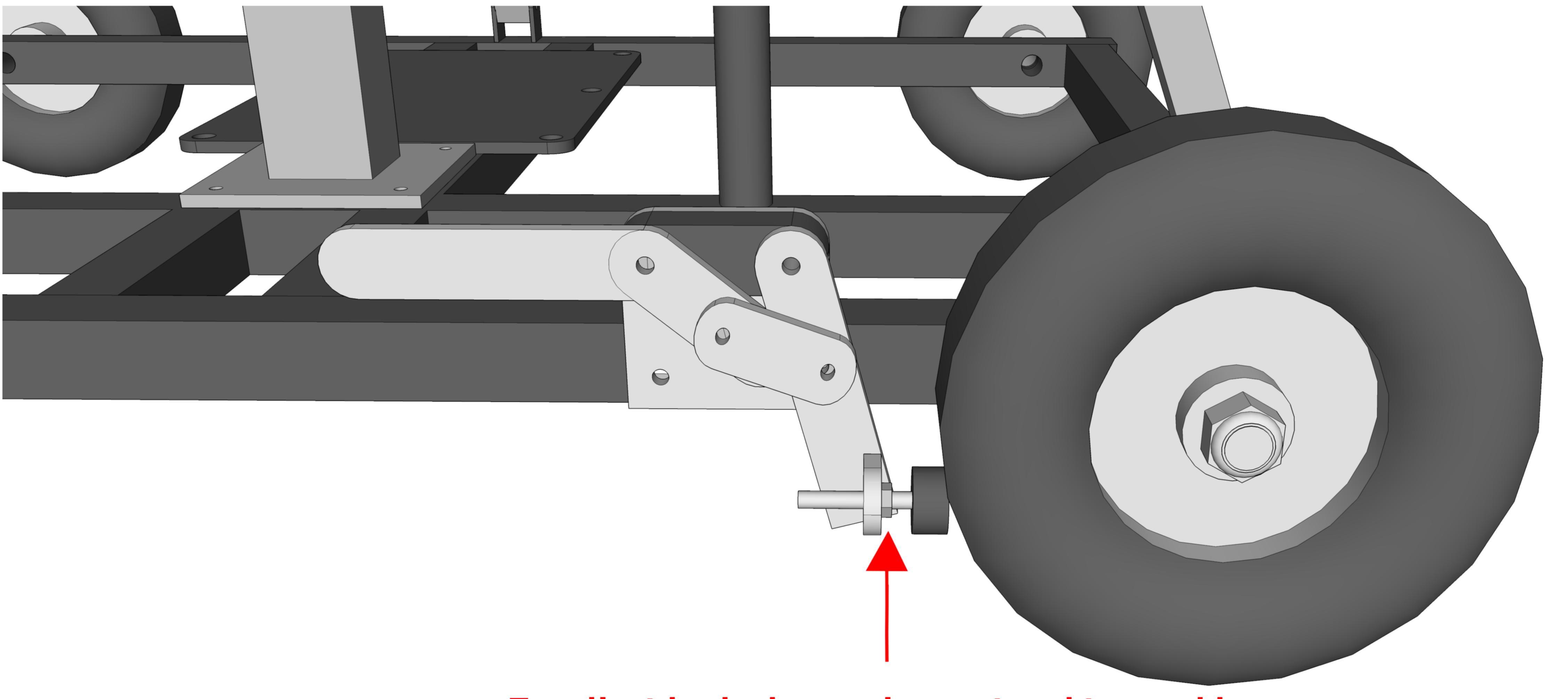
To adjust brake loosen jam nut and turn rubber bumper to increase pressure.
