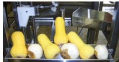
The Pre-Pack Machinery Fruit Peeler is an industrial-quality fruit and vegetable peeler built for the Fresh-Cut Produce Supplier. Its heavy-duty stainless steel material ensures a long service life and easy cleaning.
