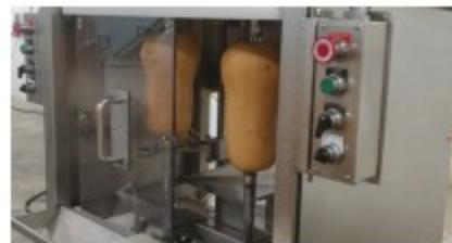
Pre-Pack Machinery's new Dually Butternut Squash Peeler satisfies today's Fresh-Cut Produce Supplier's need for higher production speed and efficiency. Its twin peeling spindles double machine production and only require a single employee's efforts.
