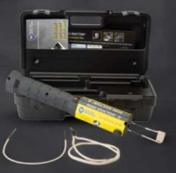
professional's choice handheld, flameless torch and leverages the power of Invisible Heat® to heat ferrous metals in seconds. Using high frequency magnetic fields, the Mini-Ductor releases corroded or frozen hardware and other metallic components from corrosion and thread lock compounds - all without the collateral damage normally associated with torches.
