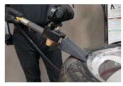
Taps directly into the tire changer's surge tank and assists in seating virtually any tire assembly.
