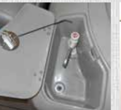
Sink Pump Faucet & Drain In Helm
