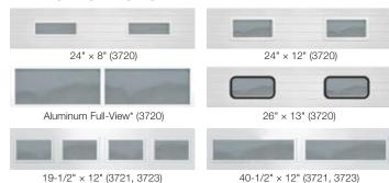
\* Intellicore polyurethane insulated option also available. Model 3720 is available with nominal insulated class and nominal insulated tempered class. Full-view section, prepainted Standard White or Chocolate; glazing options include DSB, tempered, plexiglass, insulated, insulated tempered and polycarbonate, 26" × 13" windows are available with Lexan® or plexiglass. Models 3721 and 3723 are available with DSB, plexiglass and insulated glass.
