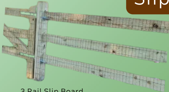
3 Rail Slip Board (Uses 1x6x10 Boards)
