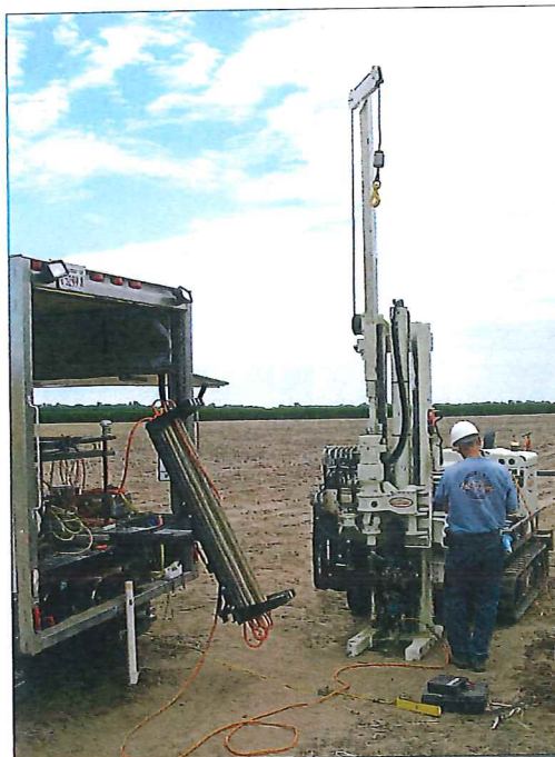
Direct Image® Subsurface Logging The 78 Series machines have been used extensively for MIP (Membrane Interface Probe), HPT (Hydraulic Profiling Tool), and EC (Electrical Conductivity) logging projects.
