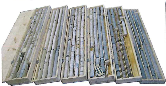
Diamond Core Drilling This 7822DT cored through rock to 150 feet using industry standard NQ wireline diamond core drilling tools. The core boxes below hold the top 115 feet of rock cores, with the top of the first core shown upper left. The site is underlain by Permian Age formations consisting of an alternating series of limestone and shale.
