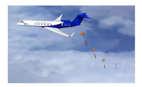
In the fascinating world of hurricane hunting, few tools are as valuable or as unique as the dropsonde. This small, tube-shaped instrument is released from aircraft directly into the heart of the storm, sending back critical data as it parachutes through swirling wind and rain. This incredible instrument that now is flown with modern aircraft through storms is a result of decades of meteorological innovation.
