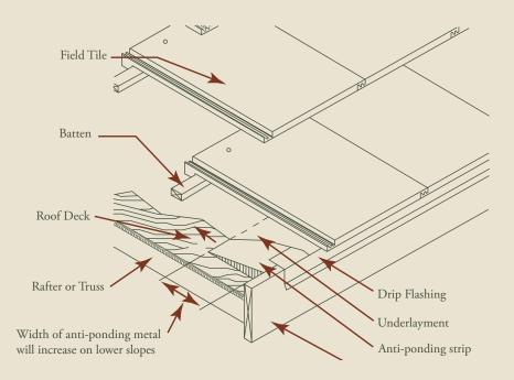
**VANDE HEY RALEIGH ROOF TILES,** designed for extreme climates, are virtually resistant to the passing of time, the ravages of weather and the hazards of fire. Our roof tile systems withstand wind-driven rain, absorb minimal moisture and defy termites, rodents and rot. Our tile meets or exceeds industry requirements for strength, water absorption, permeability, freeze-thaw, wind uplift, combustibility, dimensions and weight.
