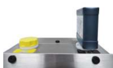
Ink bottle inserted in fill port
