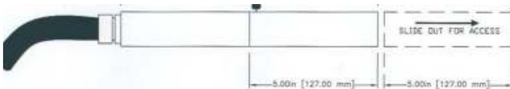
Access for Straight Printhead Umbilical Fitting (ci5200/ci5300/ci5500/ci5650)
