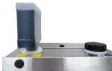
Makeup bottle inserted in fill port
