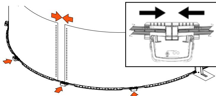
If you have carried out one of the two steps (1 & 2), you must double-check the spacing between the rails in each foot to ensure that the spacing is equal on both sides of the center of the foot.
