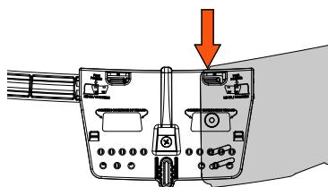
**Use the corrugation (folds or wrinkles) in the sheet to check that the uprights are vertical. Make sure the uprights are straight before screwing the ledges in place.**
