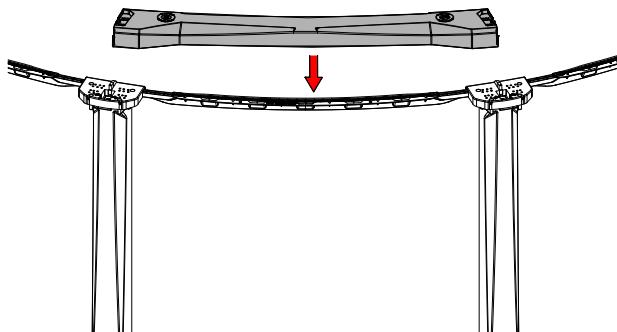
**Make sure the oblong holes on the ledge are aligned with the screw holes on the top plate.**
