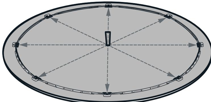
Measure each side of the foot the inside of the rail groove.
