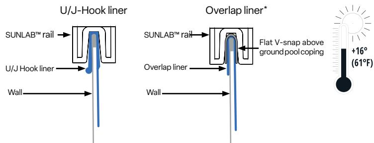
\* When installing an "Overlap" type liner, you'll need flat "V"-shaped coping to clamp the liner under the top rails. (in quantities equal to the top rails). Consult your dealer.
