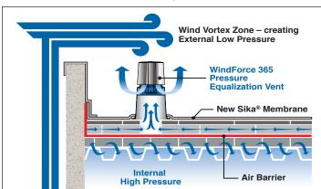
WindSmart roofs use wind currents to "vacuum-pack" the entire roof and underlying structure. Using an air tight substrate design, wind generated low pressures pull air and moisture from under the roof membrane, up through and out the strategically placed equalization vents. A suction is created, pulling the roof membrane tightly against the substrate, resisting wind uplift.
