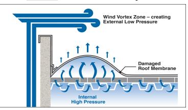
Wind currents constantly work to destroy the integrity of conventional roofs. When wind hits the side of a building, it creates an updraft. When it meets the horizontal air stream, the updraft violently tumbles, creating a horizontal vortex similar to a tornado. This wind vortex creates an external low pressure that can tear off a conventional roof assembly.
