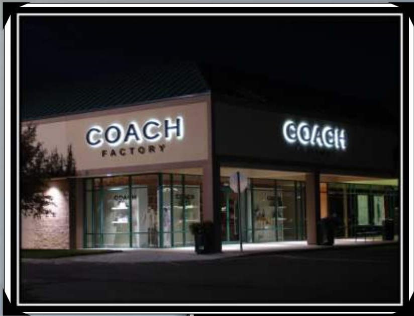
Reverse pan channel letters with halo illumination
