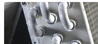
After 500 hours in a controlled corrosive environment, an all-aluminum tube sheet with an aluminum tube shows virtually no corrosion.
