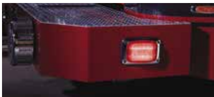
FireRay LED 6x4 (FR6C1-R) mounted on bumper with two-to-four hole conversion kit (FR6-A4HMC)
