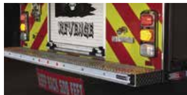
FireRay LED three-position vertical casting with FireRay LED 6x4 brake/tail/turn (FR6-BTT), arrow (FR6-ARROW), and backup (FR6-BACKUP)
