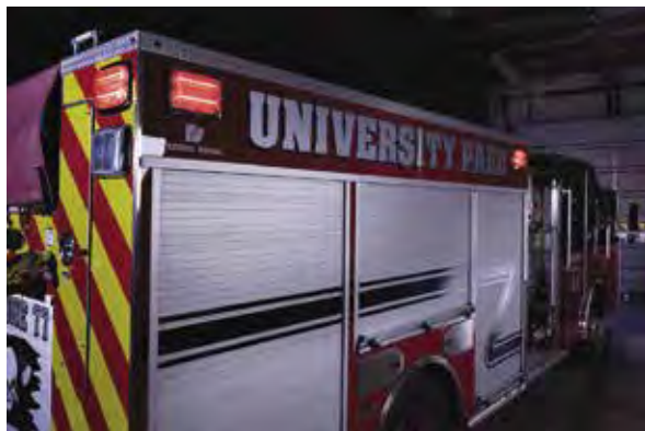
FireRay LED 9x7 (FR9C-R) mounted on side and rear of fire engine
