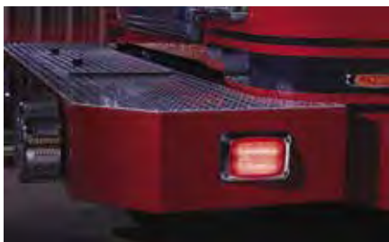
FireRay LED 6x4 (FR6C-R) mounted on bumper with two-to-four hole conversion kit (FR6-A4HMC)
