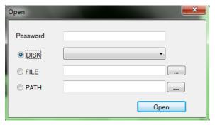
Select TF Card disk path, then click the "Open" to load and automatically play the document in the card. Clicking the ActiveX can control playing state: from left to right can realize: slow turning / stop / play (pause) / fast turning.
