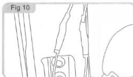
Connect the deadbolt lock with wiring harness d , blue to "+", green to "-"
