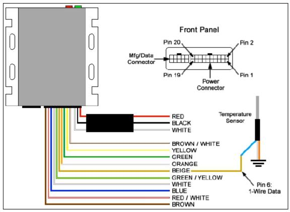
Once installed, the Temperature Sensor may be tested using the Beacon Test page in the Partner Portal, or by using the Mobile Beacon Test Tool. A fourth test has been added to the tool, which when used will send a message to the beacon to test the sensor. If the test passes, the current temperature read by the sensor is returned. If a wiring error is detected this will be reported. Or, if the sensor cannot be found, a connectivity error is reported.
