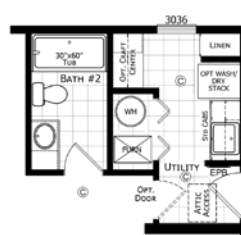
Opt. Utility Room "B"
